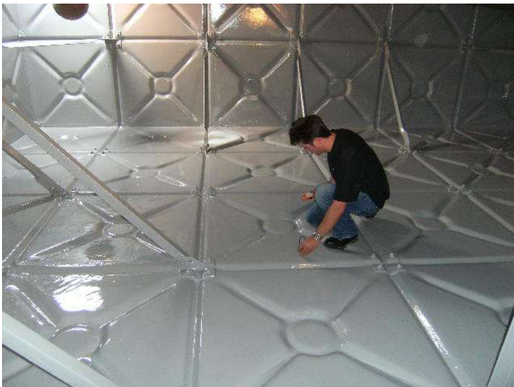
Dry Film Thickness readings were taken and recorded utilising an Elcometer 456 Microprocessor.
