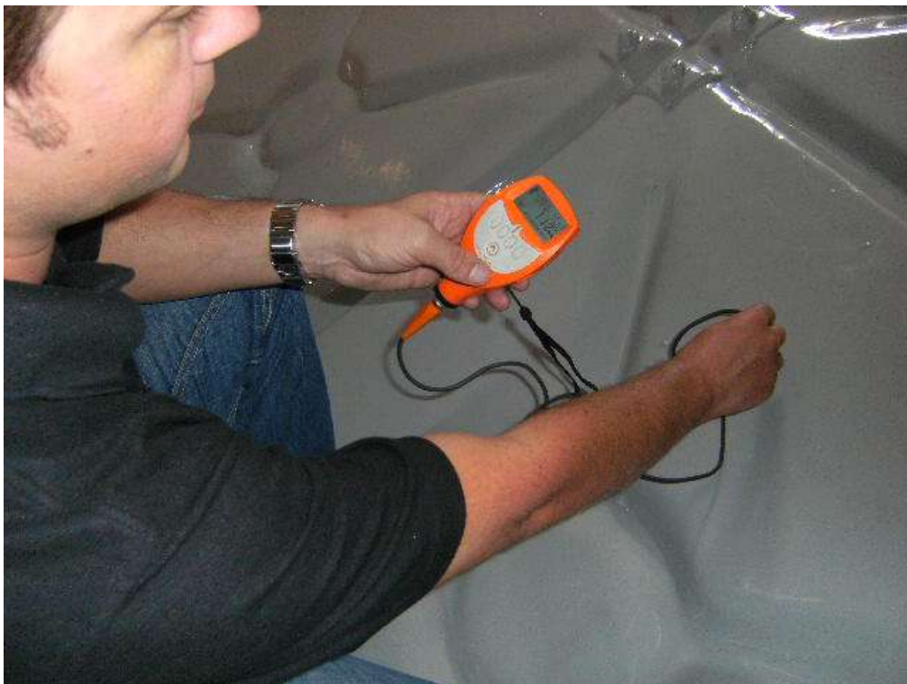
These images show the Elcometer 456 showing readings of well above the nominal 1mm (1000 Microns) thickness required.
